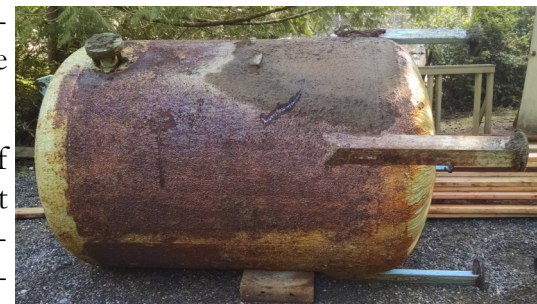
Old water filtration vessel removed from Well 2 treatment building
