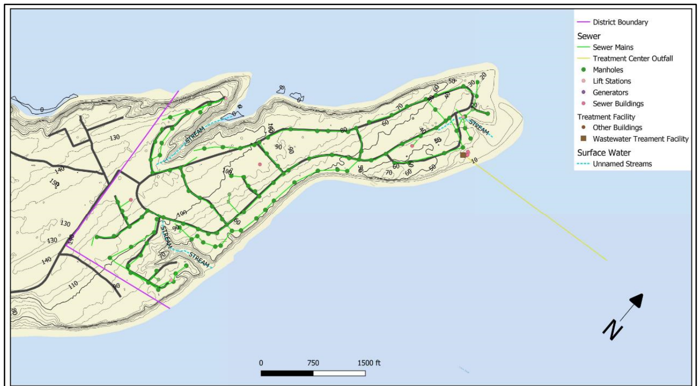
Figure 2-1. Existing Sewer System
